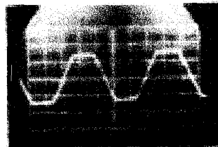
Amplzilla at clipping (240 Watts R.M.S.) at 20 KHz - Note practically zero recovery time.
